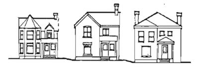
**Avoid** -Introducing incompatible facade patterns that upset the rhythm of openings established in surrounding structures. Glass walls and window and door shapes and locations shown in the example are disrespectful to the adjoining buildings.
